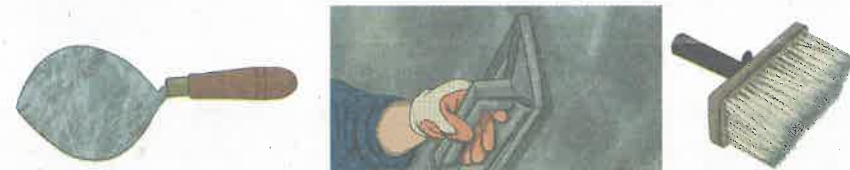
Trowel/Thappa/Karni: It is used to apply and flatten the plaster.
